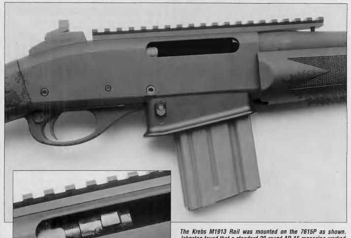
Johnston found that a standard 20-round AR-15 magazine worked well for its compactness. (inset) Like its Model 7600 sibling, the Remington 7615P uses a two-lug rotating bolt for strength and reliability.
